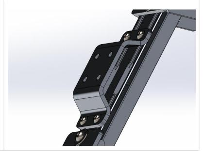
3. Locate the channel on the cross rail and insert the square nuts.
