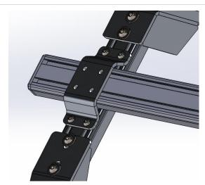
5. Use the 1/4"-20 screws to secure the cross rail to the claw bracket. Repeat on the other side.
