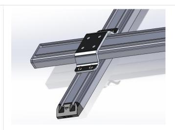
5. Use the 1/4"-20 screws to secure the cross rail to the claw bracket. Repeat on the other side.
