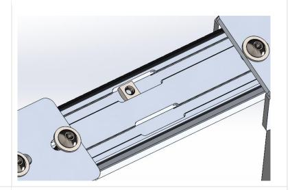
2. Mount the bracket using the 1/4"-20 screws.
