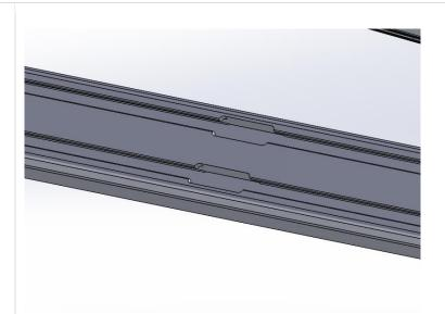
4. Slide the cross rail so that it aligns with the claw bracket.
