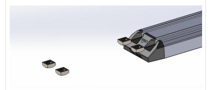
2. Mount the bracket using the 1/4"-20 screws.
