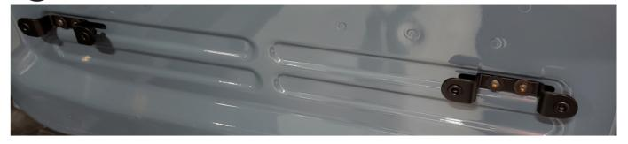
Loosely attach the backing plate to the molle panel with the 3/8 bolts, washers, and spacers as shown in Figure 3.
