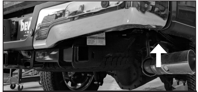
Figure 1: Location of factory wire harness.
