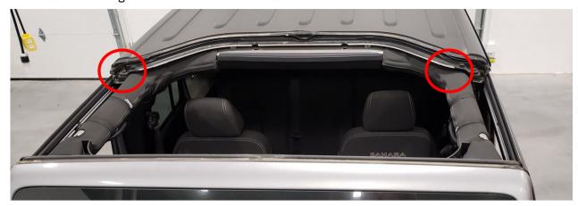
2. Place the Sky View roof panel on the top of the vehicle. Do not remove the protective film from the clear roof panel until the installation is complete. Only peel back the protective film as far as necessary to install the clear roof panel.
