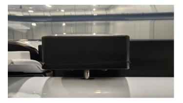
8. The rubber damper should be placed between the handle and the roll bar to prevent scratching your factory paint. It's important to note that a slight gap between the roll bar and the screw plate is entirely normal, do **not** over-tightening the components.
