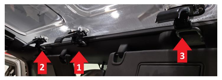
6. Starting at the rear of the vehicle, slowly tighten the hand bolts in the order shown below. Do not over tighten.
