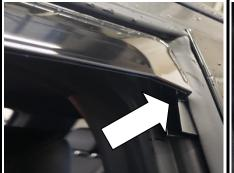
After installing the visor, insert the channel spacer into the channel as shown. See the back of these instructions for application-specific spacer locations.
