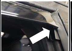
After installing the visor, insert the channel spacer into the channel as shown. See the back of these instructions for application-specific spacer locations.
