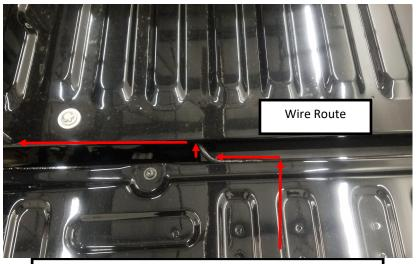
7. Feed LED emblem wires to driver's tail lamp harness. Follow existing harness coming out of tailgate. Route the wire under the vehicle, behind the bumper, and up into the tail lamp cavity. Protect the wire with split loom or abrasion resistant sleeving.
