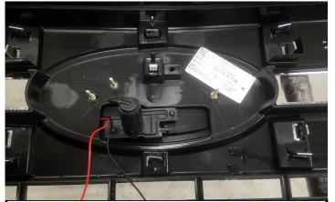
9. Install emblem onto grille with provided (3) flange nuts. Tighten with 8mm wrench, being careful not to overtighten.
