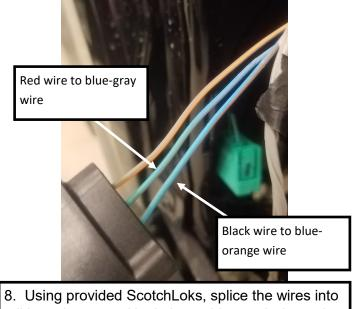
8. Using provided ScotchLoks, splice the wires into tail lamp harness. Hook the emblem red wire to the blue gray wire, and the emblem black wire to blue orange wire.
