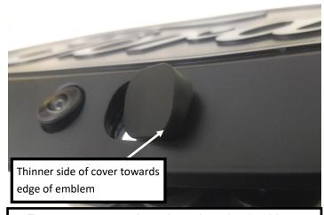
8. Front camera equipped trucks: Apply 3M tape to back of included washer cover. Peel backing off and press onto factory washer cover. Make sure orientation is correct!
