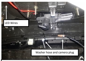
10. Reconnect any plugs for camera system and washer nozzle, if applicable. Feed LED emblem wires towards top of grille to finalize connections. Push grille into place, but do not install fasteners until emblem has been fully installed and tested.
