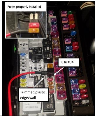
12. Remove Fuse #34 (10A fuse). Insert it in Add-A -Fuse tap and install provided 5A fuse on the wire side of Add-A-Fuse tap, as pictured. Install assembly into Fuse #34 slot. Some trucks may require use of wire cutters to trim of plastic edge in fuse box to allow wire to pass out.
