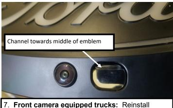
7. Front camera equipped trucks: Reinstall nozzle cover, ensuring proper orientation. Needle nose pliers may be needed to pull nozzle arm through opening when installing nozzle cover.
