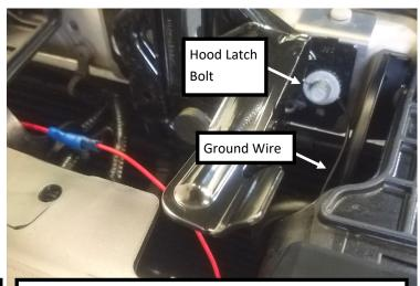
13. Connect Add-A-Fuse harness to red wire from LED emblem. Strip  $\sim$ 1/2" of insulation from black wire, and ground to chassis. For example, loosen (do not remove) the 10mm bolt holding hood latch enough to wrap black ground wire around bolt. Tighten bolt, making sure wire is secured.
