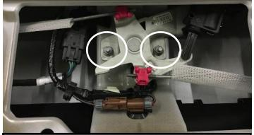
2. Remove (2) 10mm bolts and shift latch assembly out of the way. This allows for better access to the back side of the emblem.
