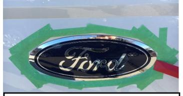
3. The emblem is held by 2 plastic clips and adhesive tape. Carefully pry on emblem and push the clips from inside the tailgate. **BE CAREFUL NOT TO DAMAGE THE PAINT OR SHEET METAL.**
