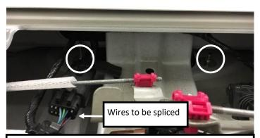
5. Install the emblem into the tailgate using the provided flange nuts. **Be careful not to overtighten the fasteners and damage the tailgate.**
