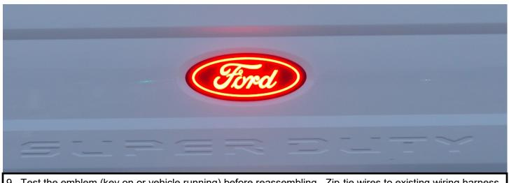
9. Test the emblem (key on or vehicle running) before reassembling. Zip-tie wires to existing wiring harness. Keep the wire clear of sharp edges and from interfering with latch mechanism.
