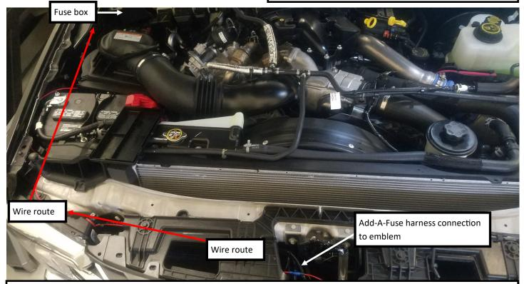
11. Connect the Add-A-Fuse tap to the LED emblem and route it to the fuse box. Be careful to avoid sharp edges and moving parts. Zip-tie wire in place when installation is complete.
