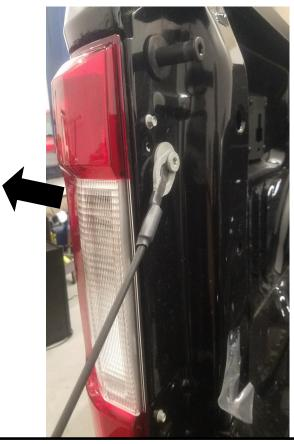
6. Remove (2) 8mm bolts from driver's tail lamp. Pull out on tail lamp (away from fender) to remove from vehicle.
