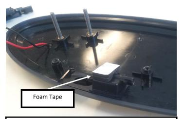
6. **Front camera equipped trucks:** Apply 3M foam tape to back of camera to prevent vibration in housing. Reinstall camera and washer nozzle mounting assembly using original T25 torx screws.
