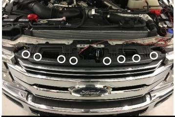
2. Once cover is removed, remove the top 8 grille screws with 10mm wrench (location shown above).
