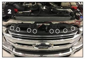
Once cover is removed, remove the top 8 grille screws with 10mm wrench (location shown above).
