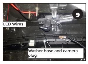
Reconnect any plugs for camera system and washer nozzle, if applicable. Feed LED emblem wires towards top of grille to finalize connections. Push grille into place, but do not install fasteners until emblem has been fully installed and tested.
