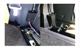
9. The driver box can now be wired to dash mounted switches and 12V power inside the cab. Power can be grabbed from near the cab fuse box or a cigarette outlet depending on your truck model. See table on next page for wire functions.
