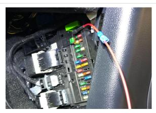
10. The workblade cab mount can also be used with the OPTIONAL wireless remote. Red= +12V, Black= Negative, Blue= Switched power (A), Orange, green and grey = Momentary switched ground (B,C,D) see wireless remote instructions for more details.
