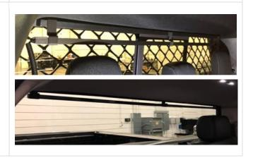
8. Using 3M tape or zip ties mount the driver box behind your rear seat.
