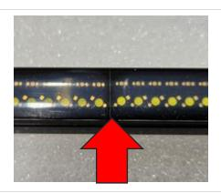
5. The kit comes with four 10.25" u-channel shroud pieces. These clip onto the light bar to eliminate cab glare. They are held in place by compression. Slide the U channel towards the center so there are no gaps between each u-channel.
